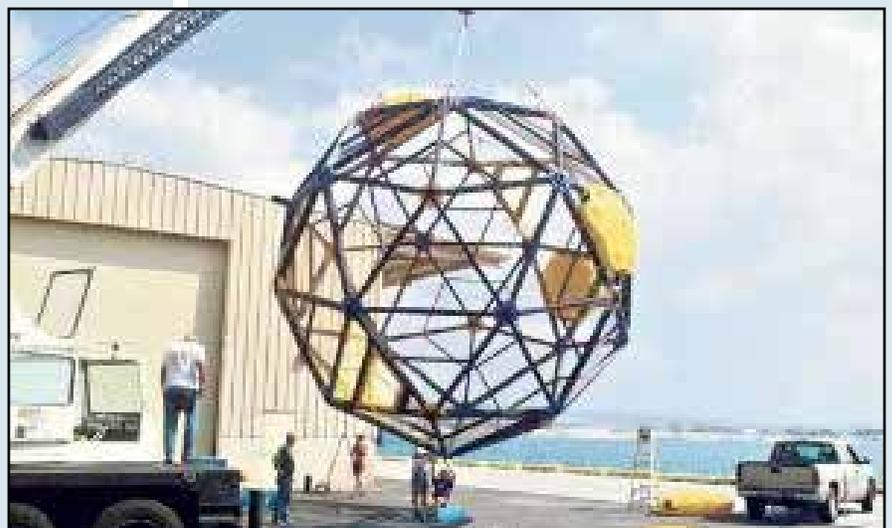
The Aquapod 212 submersible cage used to study the feasibility of free-floating fish farms. The net pen is 27 feet in diameter and made from structural-plastic framing covered with brass-mesh netting. Credit: [www.staradvertiser.com](http://www.staradvertiser.com)
